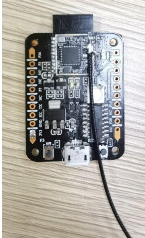
Figure 7 schematic diagram of antenna test prototype
